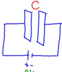
Think of a capacitor like a spring. When the spring is stretched, it stores potential elastic energy similar to how a capacitor will store electric potential energy.
